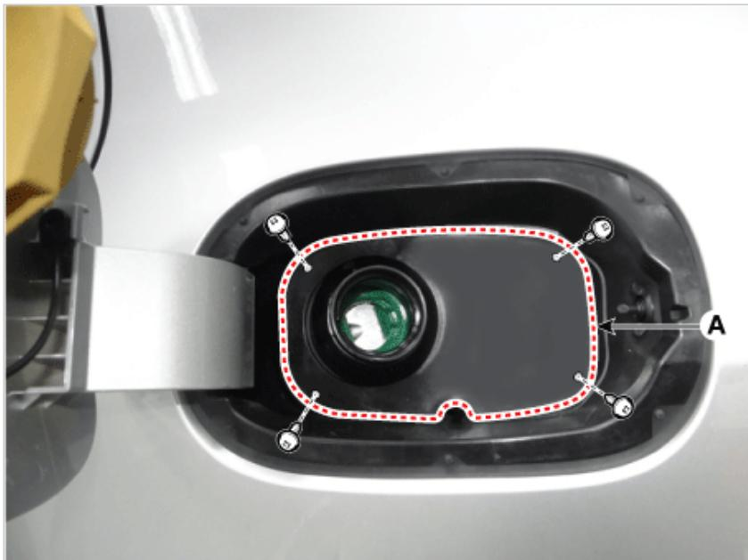
3. Remove the fuel filler door fixing pin (A).
