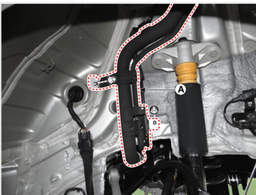
5. After loosening the mounting bolts, remove the fuel filler door (A).
